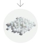
These flakes are melted into chips and blown into polyester staple fibre.
