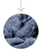
The fabric is shredded in a spinning mill and blended with virgin organic cotton.
